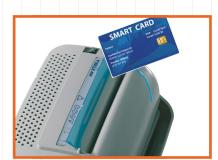
As per NSA/CSS requirements, cards must be inserted at a 45 degree angle, for proper data sanitization
